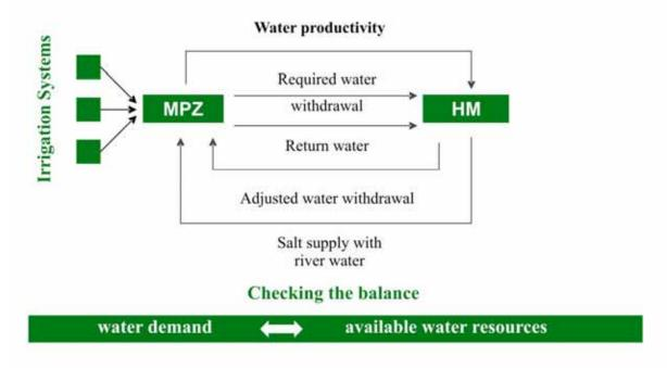
Figure 4.7 Links between the Hydrological Model (HM) and the Planning Zone Model (MPZ)
